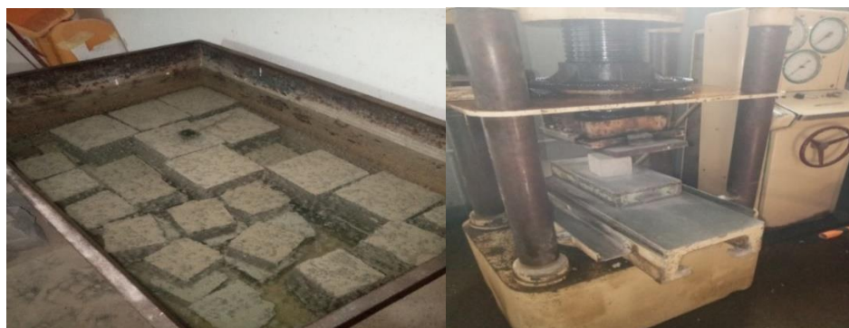
Plate 1. concrete curing and crushing
